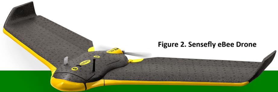
Figure 2. Sensefly eBee Drone
